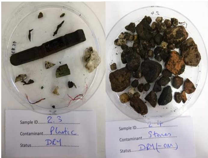
Sampling and testing of physical contaminants in PAS composts and digestates
